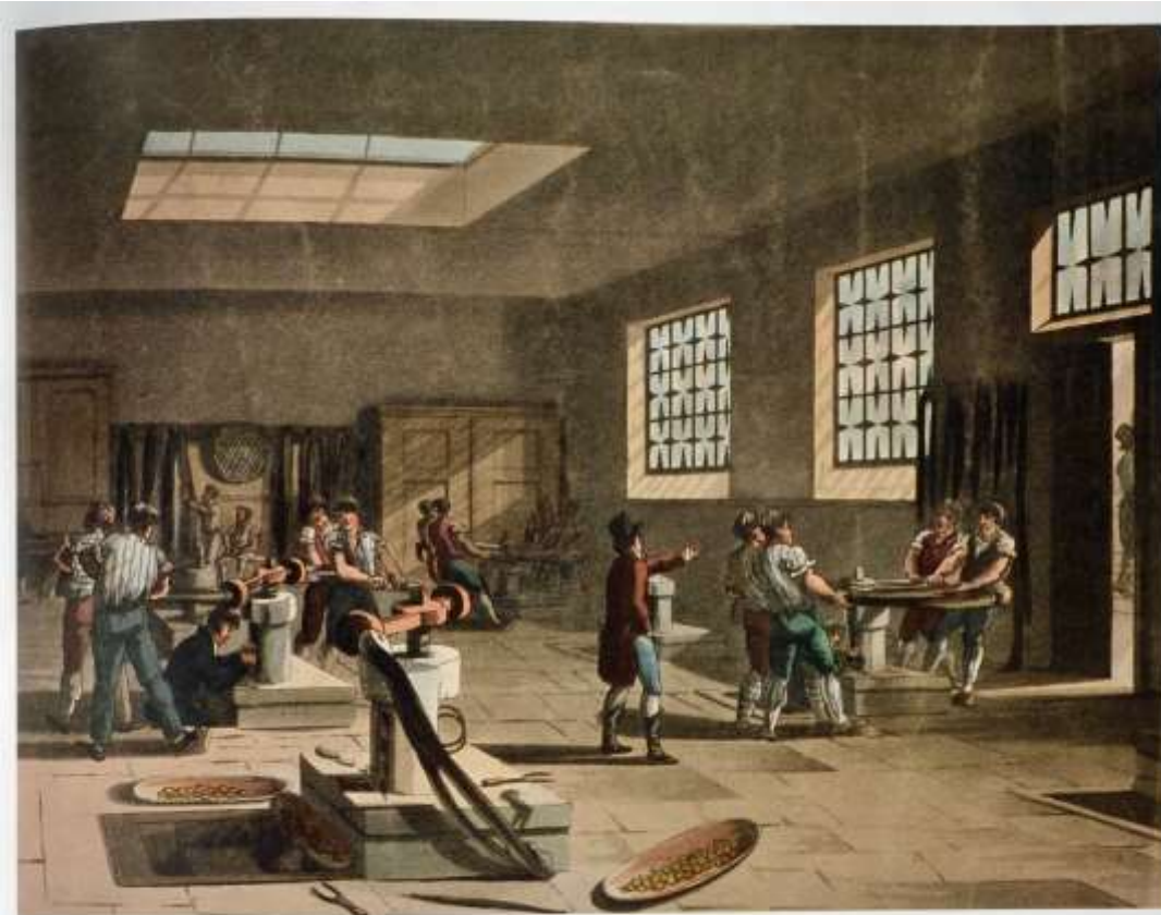
213. Capstan Fly Presses (left) and Wheel Presses (right) at the Royal Mint. From Rudolph Ackermann's Microcosm of London , Vol. II, Plate 55 (1809).
